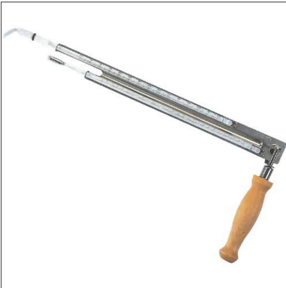
Figure 3: Sling Psychrometer (US Weather Bureau type)
